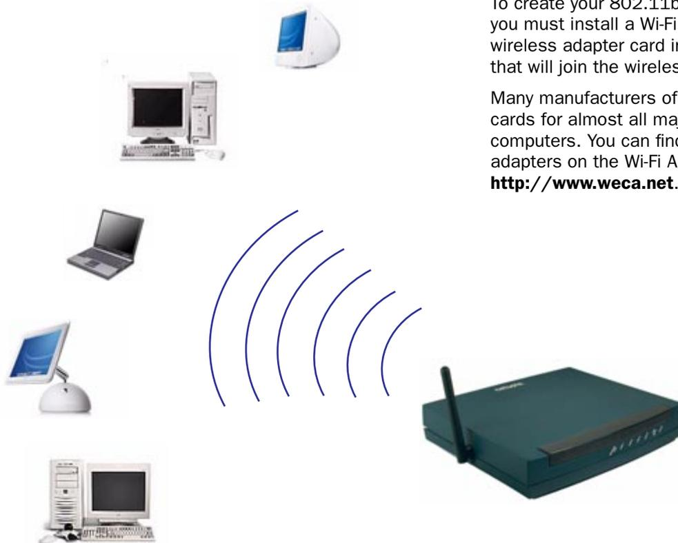
To create your 802.11b wireless network you must install a Wi-Fi CERTIFIED™ wireless adapter card in each computer that will join the wireless LAN.
