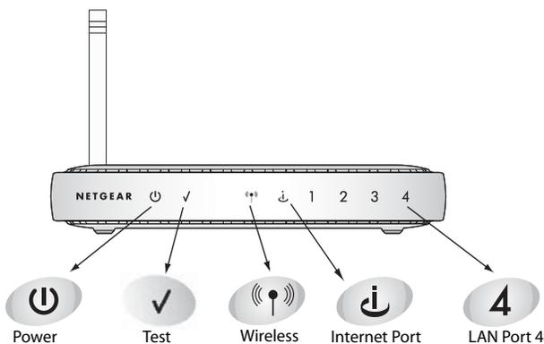
**Figure 2-1: WGR614 v6 Front Panel**
